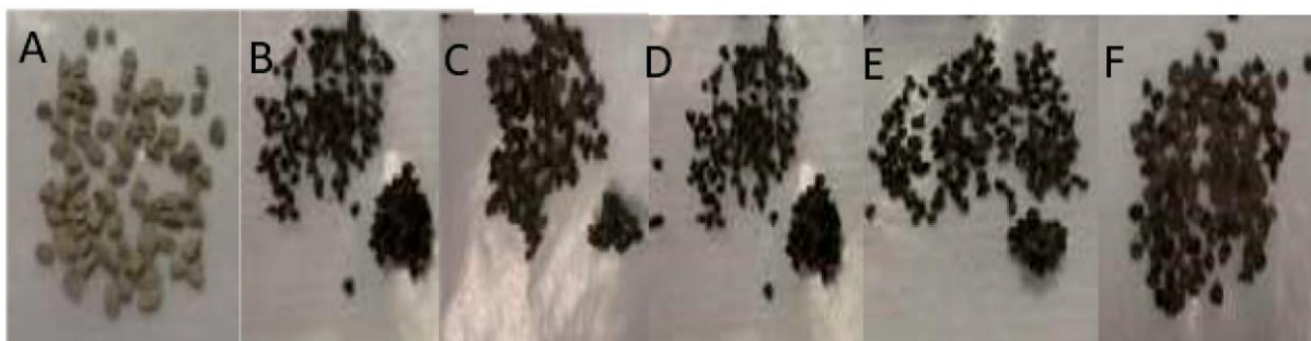
Figure 5: External Appearance of (A) Fresh and (B–F) Reacted Catalyst Samples at 500, 550, 600, 650, and 700 °C.
